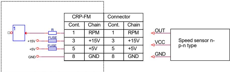
Figure 11. Speed sensor connection socket
