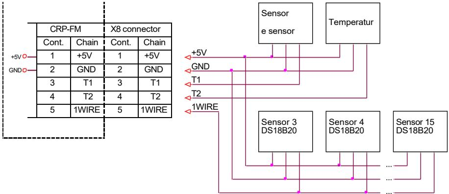
Figure 14. Temperature sensor connector
