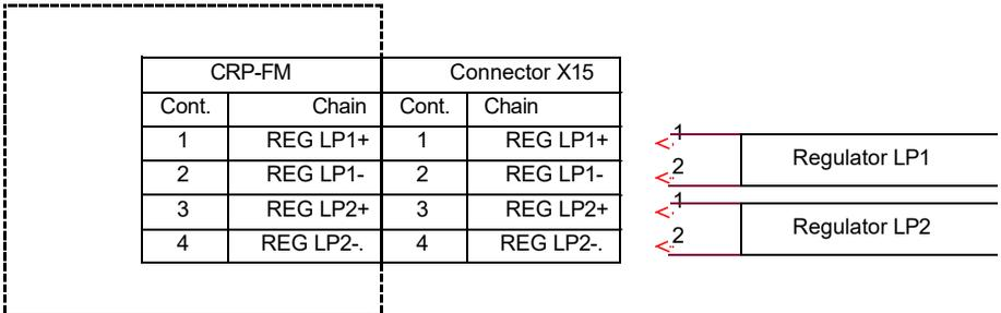
Figure 23. Connector X15, pump controller valve control outputs
