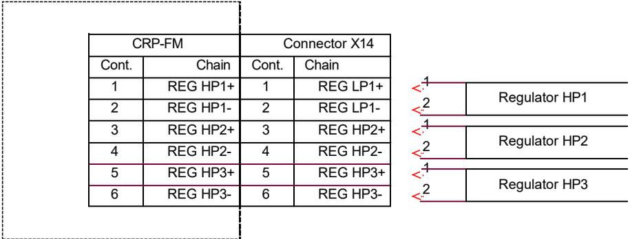
Figure 22. Connector X14, rail pressure regulator control outputs
