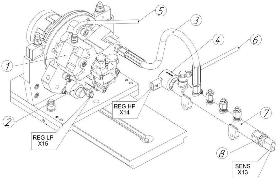
Figure 6.Pump and rail connection diagram
