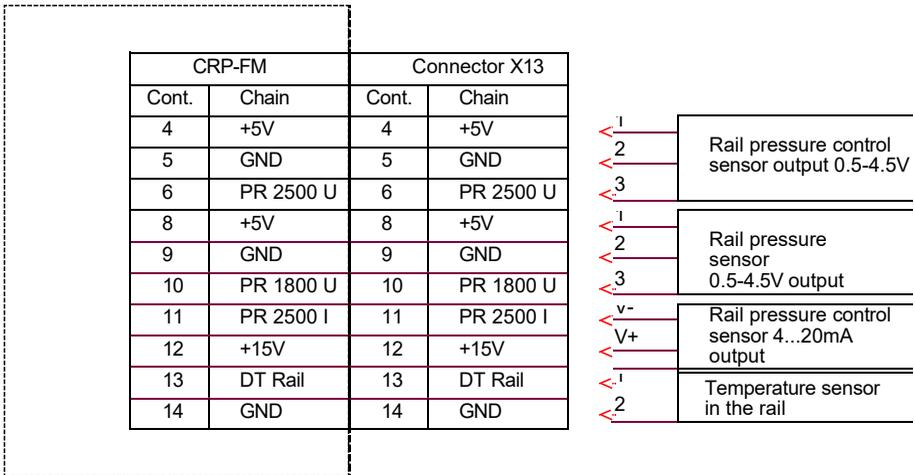
Figure 20.Connector X13, high rail pressure measurement
