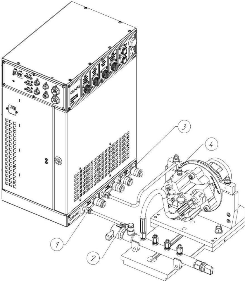
Figure 7. Hydraulic connection of the pump to the meter
