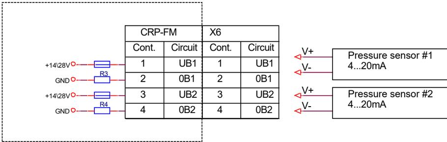
Figure 12. Sensor connection socket with 4-20mA output
