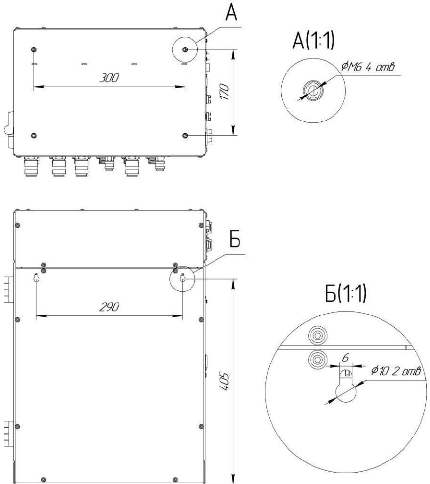
Figure 25. Mounting dimensions
