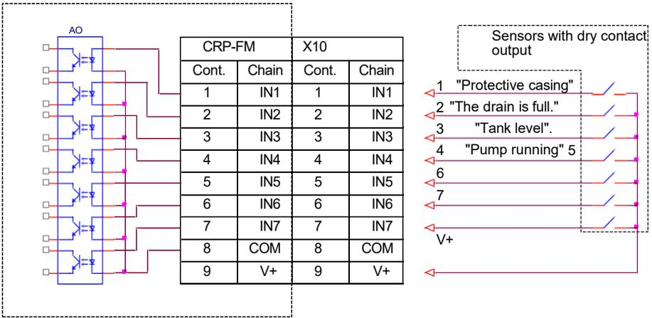
Figure 16. Connector for connecting actuator sensors.
