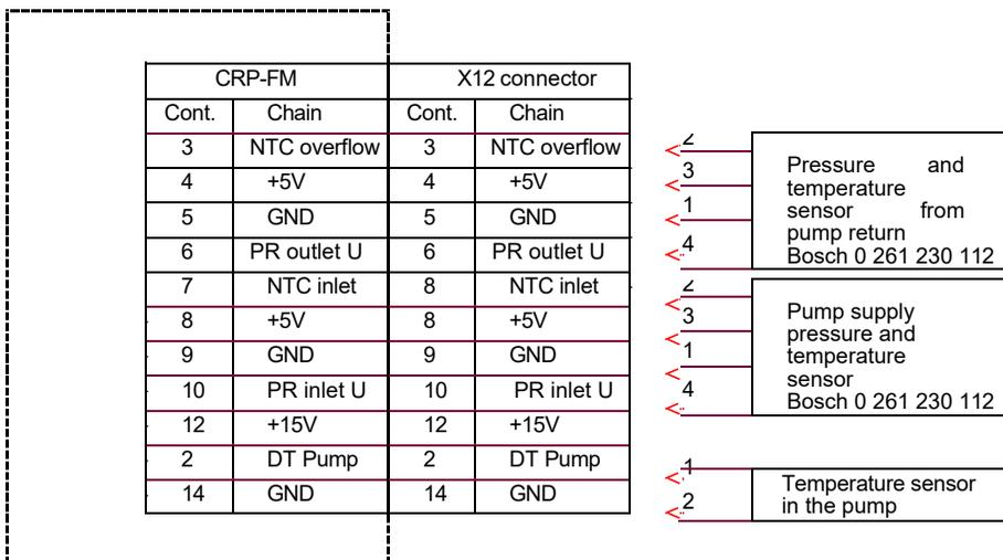
Figure 19.Connector X12, pump inlet pressure measurement and return line pressure of the pump under test
