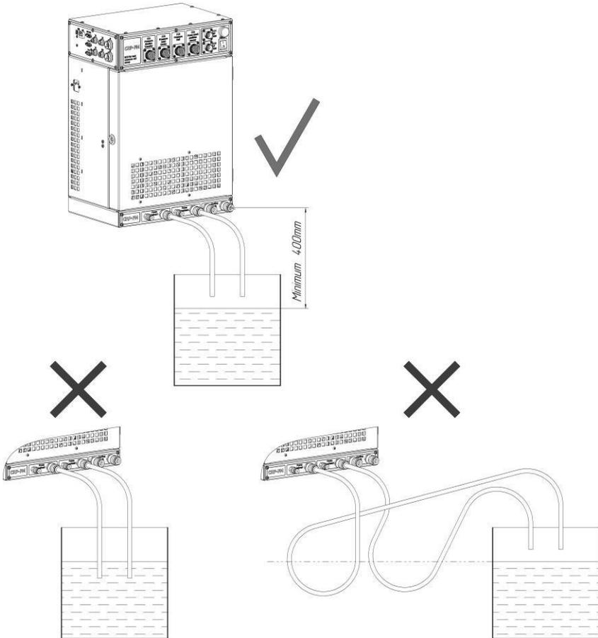
Figure 9. Restrictions on the connection of the measured liquid return flow
