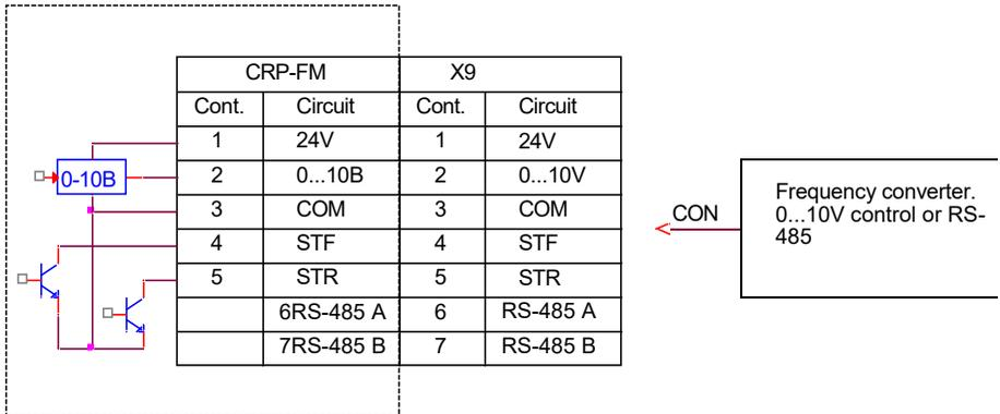
Figure 15. Frequency converter connection socket
