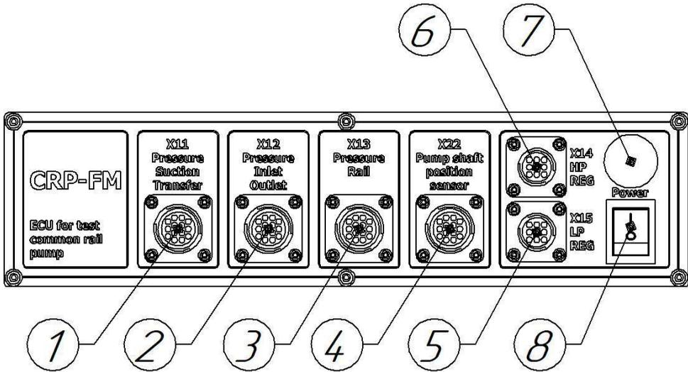
Figure 4. Electrical connection panel to the pump
