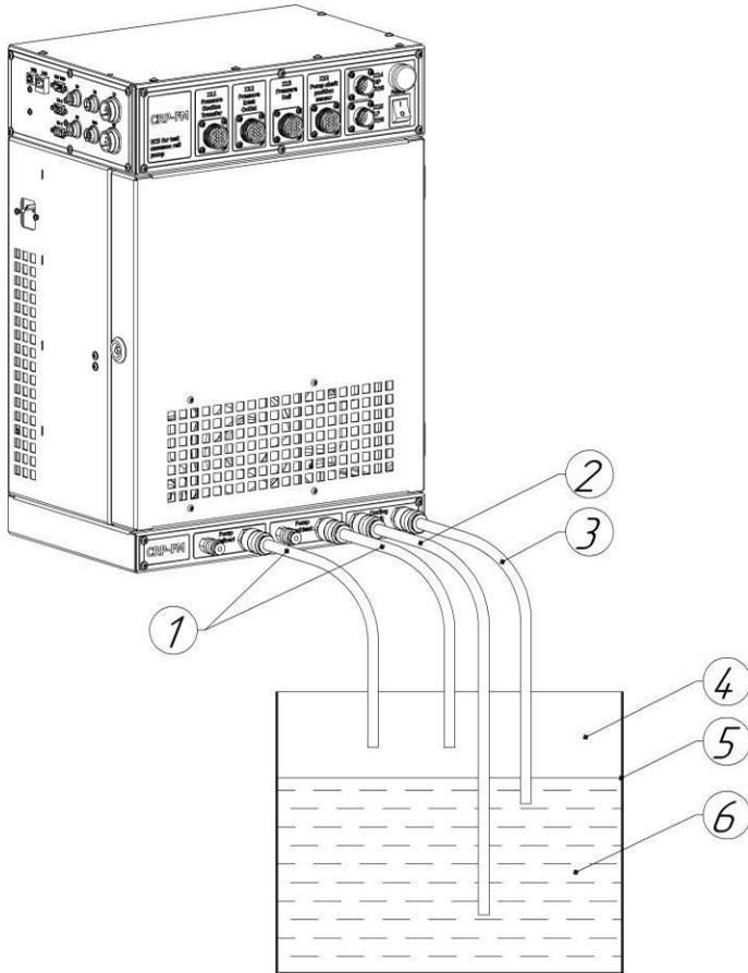
Figure 8. Hydraulic connection of the meter to the test bench
