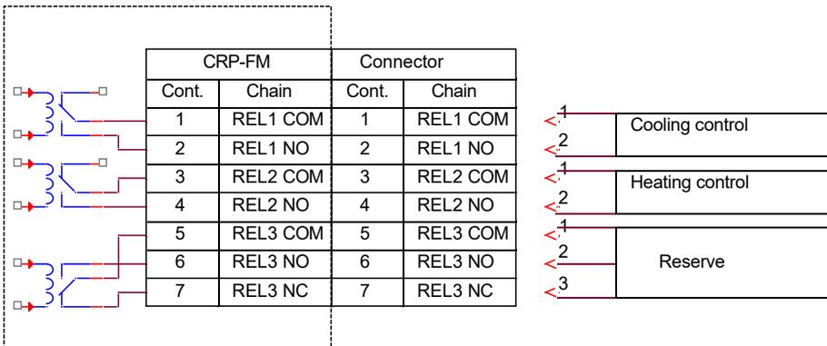
Figure 13. Burner control/cooling connection
