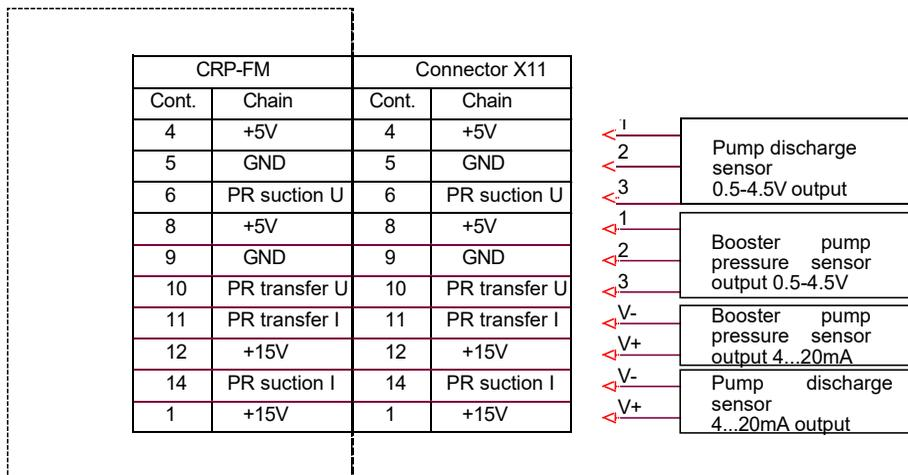
Figure 18.Connector X11, supply pump pressure measurement and vacuum system measurement of the pump under test
