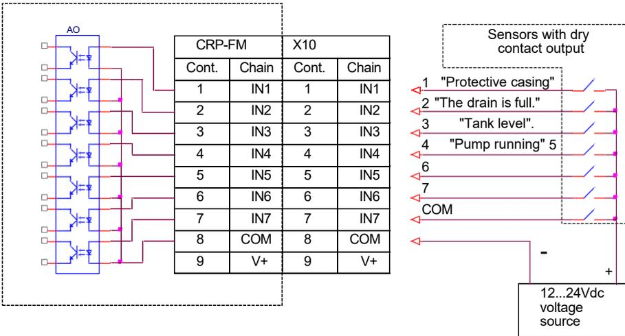
Figure 17. Connector for connecting actuator sensors.
