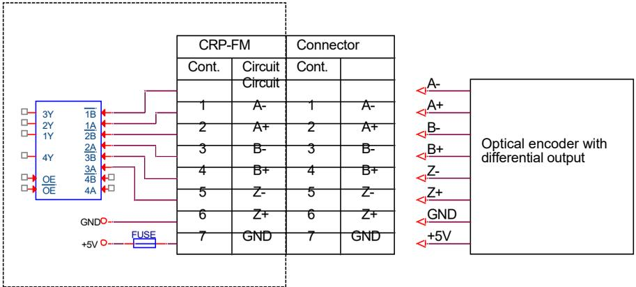
Figure 10. Encoder connection connector
