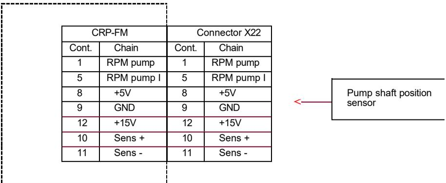
Figure 21.Connector X22, shaft position sensor for pump under test
